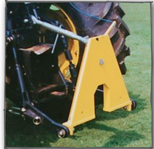
Delta-hook tractor rapid hitch.
